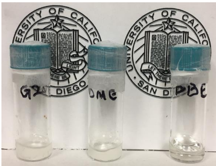
Fig. S1. Photos of selected electrolytes. Photos of 2 M LiFSI dissolved in G2, DME or DBE after storage at -60\text{ }^{\circ}\text{C} overnight.
